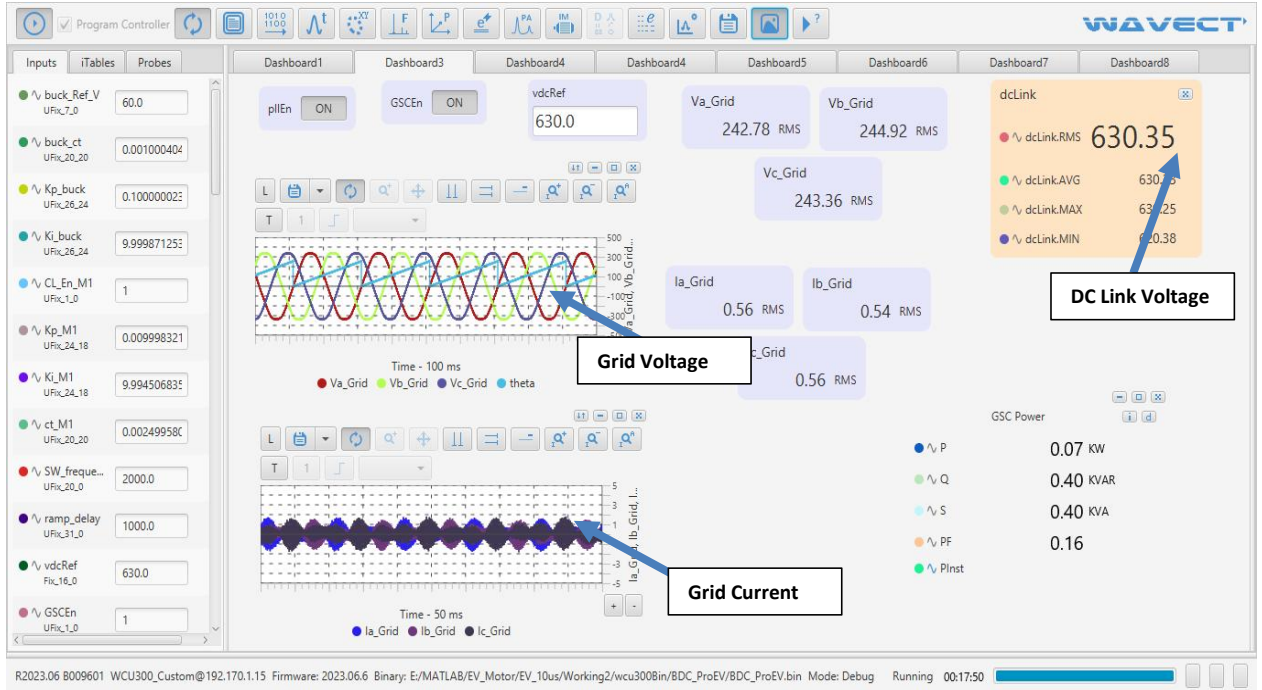
Figure 12: Grid Side Converter Panel.
