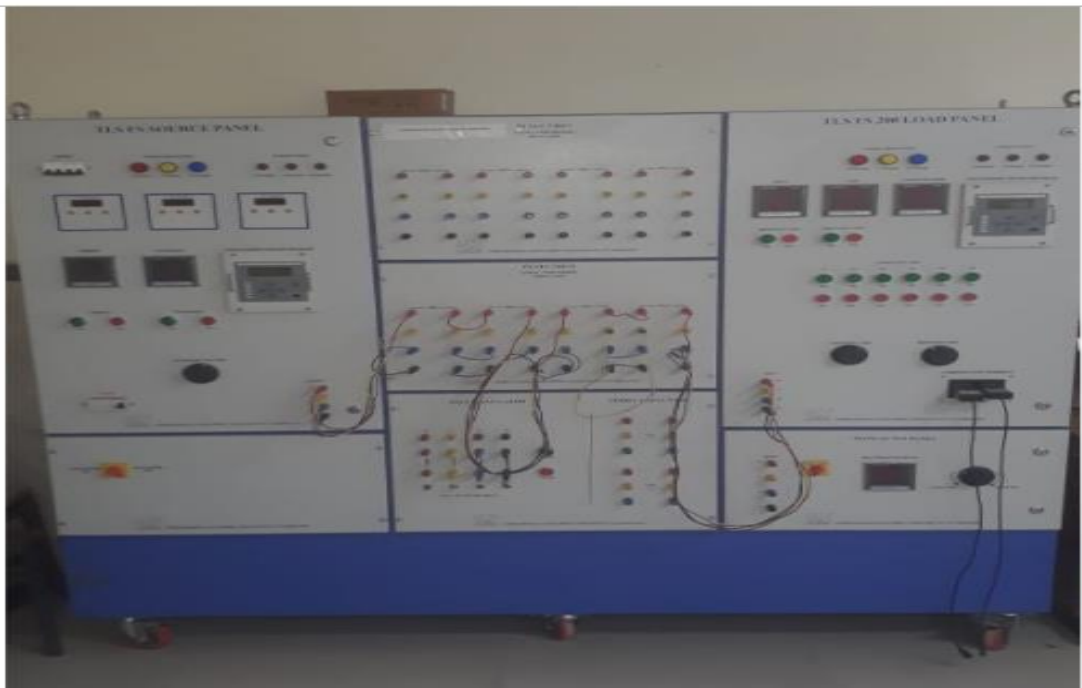
Pictorial view of transmission line Simulator
